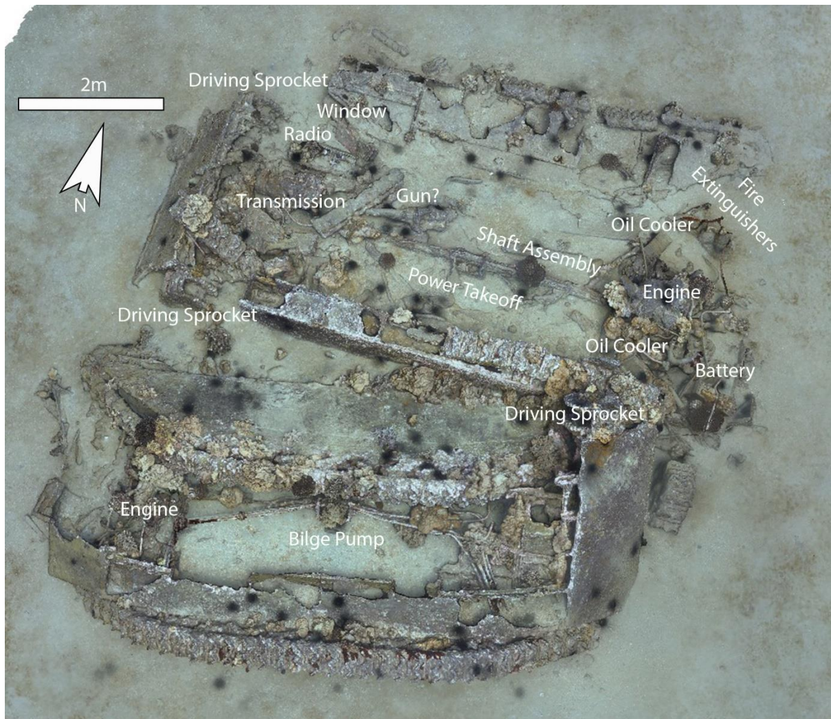
Figure 3. 3D model of previously unrecorded LVT-2 wrecks in Mā'alaea Bay. Identifiable components are labeled (courtesy ECU/UCLA).
