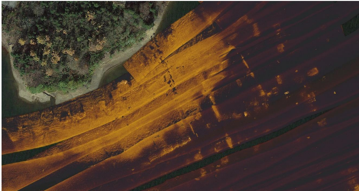
Figure 3 A Side Scan Sonar Mosaic Image overlayed; Showing the Outlines of the Village in Reflections (image provided by the research team)
