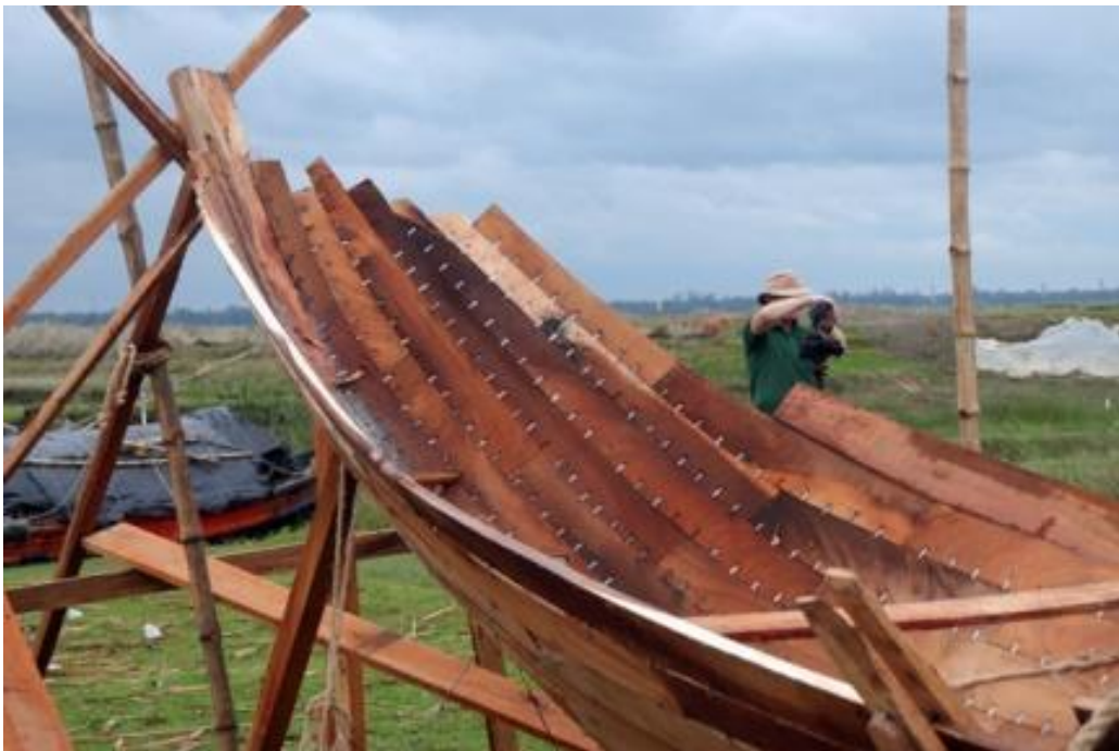
Figure 2. Hull planking. Planks used in the hull planking are run parallel to the keel. Smaller planks are used in the stem and stern region.
