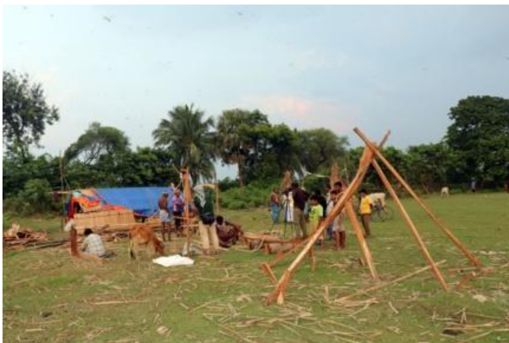
Figure 1. Entire keel after erection. Various support systems are used to hold the keel in its position.
