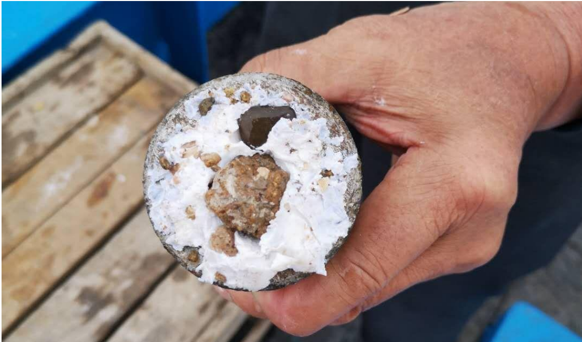
Figure 1: Detected Seabed Topography and Sediment Using a Sounding Lead
