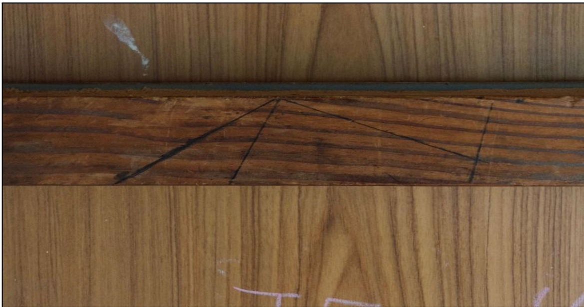
Figure 6: Angles drawn on the wall of the shop, used by Mr. Hiroshi Murakami in building the isobune in Iwate.
