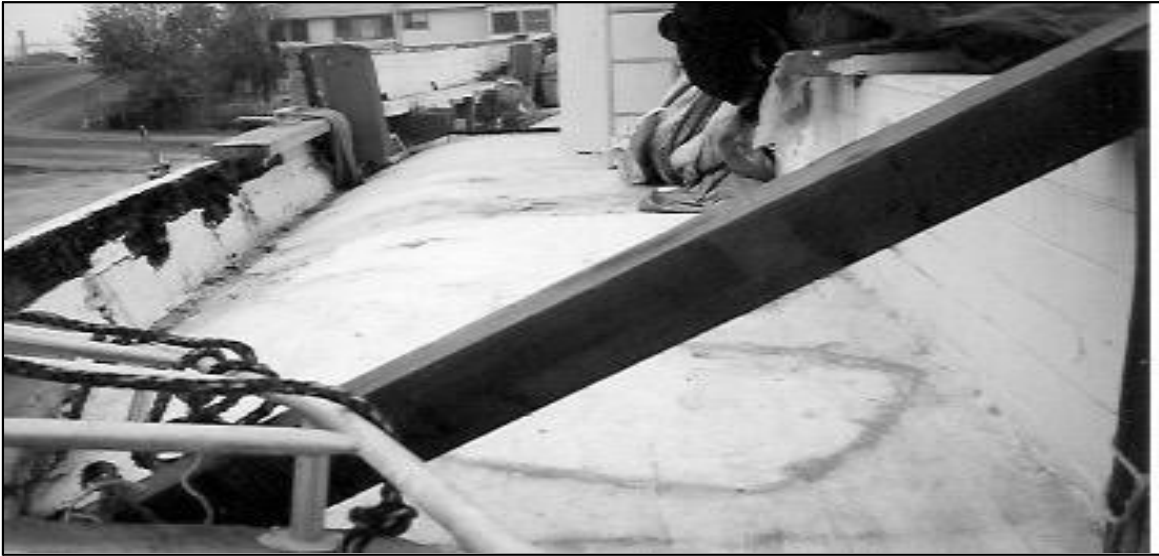
Figure 3: Self-draining Deck of the Free China.
